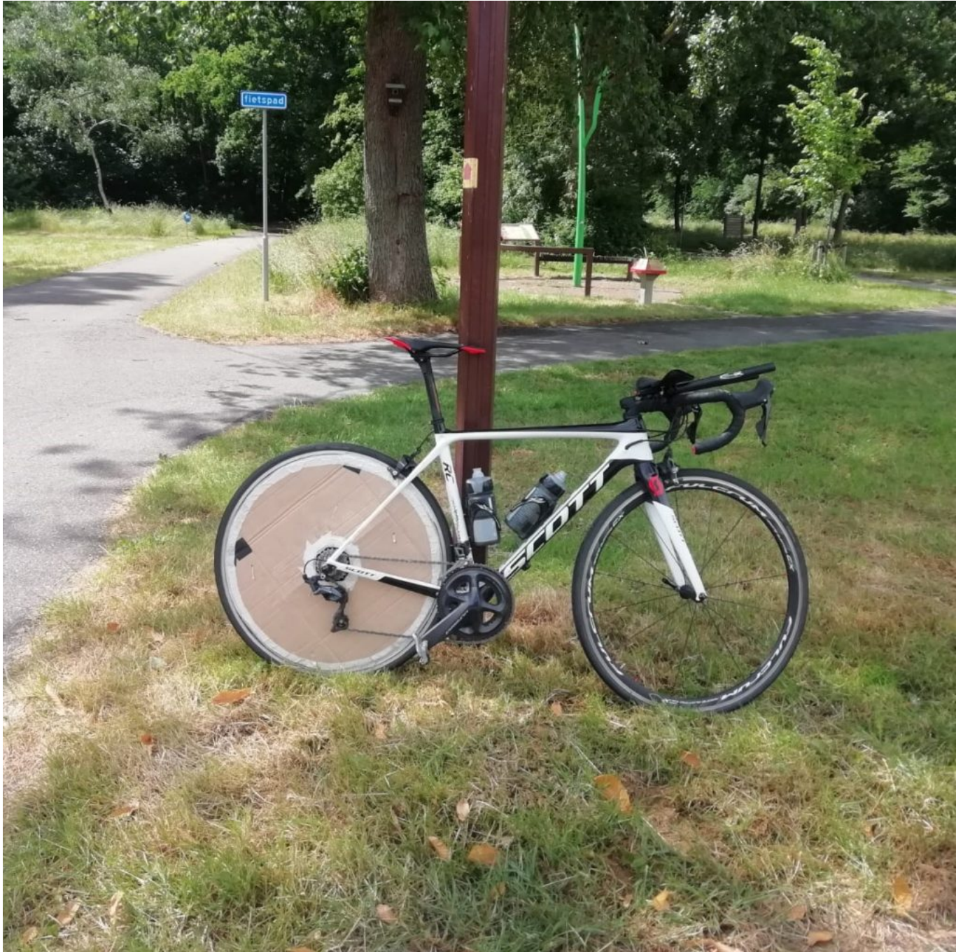
Condition III: Aero + self-made disc wheel from cardboard
