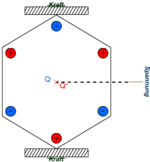
The piezoelectric effect. [Spannung] german for voltage; [Kraft] german for force
