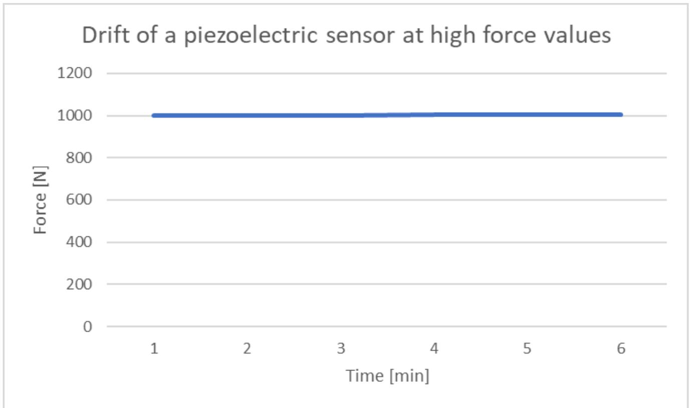
Effect of drift at small and at high force values: At a measurement of 1000 N, longer measurement times are possible because the relative error remains small; at smaller forces, the effect of drift is more noticeable.
